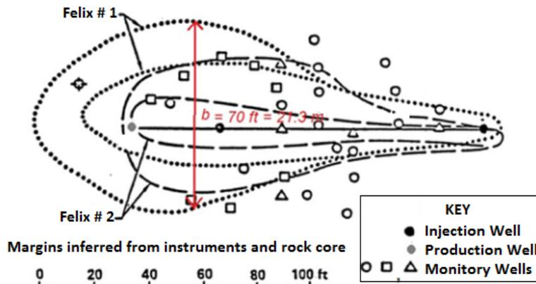
Figure 6. Possible gas cavity configuration plan view and the measurement of 'b', derived from the Felix 1 and 2 experiments [9]
