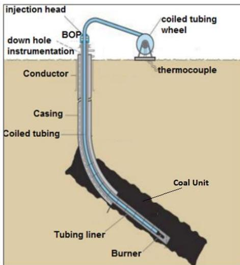
Figure 2. General components for directional drilling [1]
