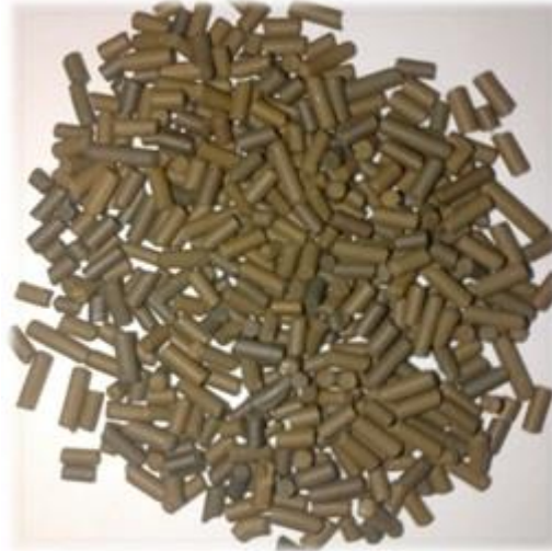
Figure 2 Rod-shaped proppant typical cylindrical shape
