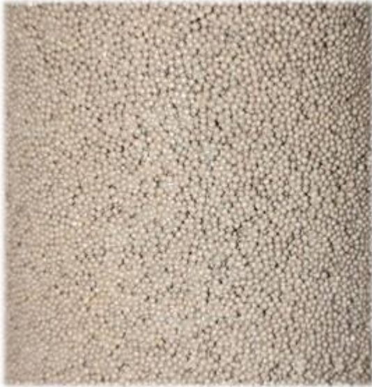
Figure 1 Resin-coated proppant after complete curing process
