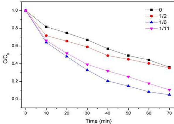
Fig.5. Photocatalytic performance of samples towards the degradation of RhB
