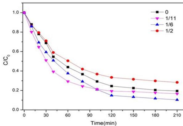
Fig.7. Photocatalytic performance of samples towards the degradation of TC
