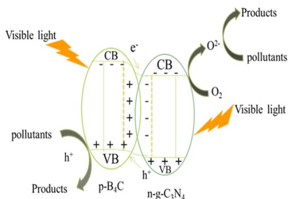
Fig.10. Possible photocatalytic mechanism over  $\text{B}_4\text{C}/\text{g-C}_3\text{N}_4$  under visible light irradiation
