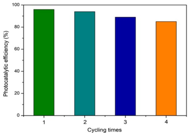
Fig.8. Repeated experiments on the photocatalytic degradation of RhB by B<sub>4</sub>C/g-C<sub>3</sub>N<sub>4</sub> (1/6)
