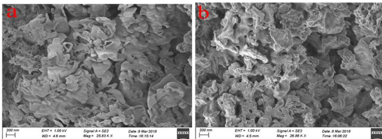
Fig.2. SEM patterns of (a)  $g-C_3N_4$  and (b)  $B_4C/g-C_3N_4$ (1/6)
