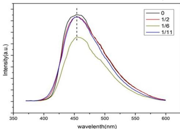
Fig.4. PL spectra of the photocatalysts excited at the wavelength of 325 nm
