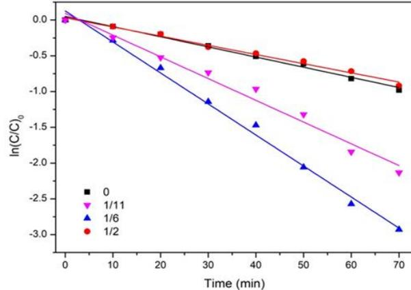
Fig.6. Kinetic rate constants of RhB degradation over B<sub>4</sub>C/g-C<sub>3</sub>N<sub>4</sub> composites
