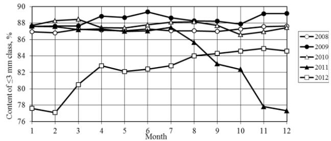
Fig. 4. Variation in the content of the  $\leq 3$  mm class in the coal batch at coke batteries 1–4 between 2008 and 2012
