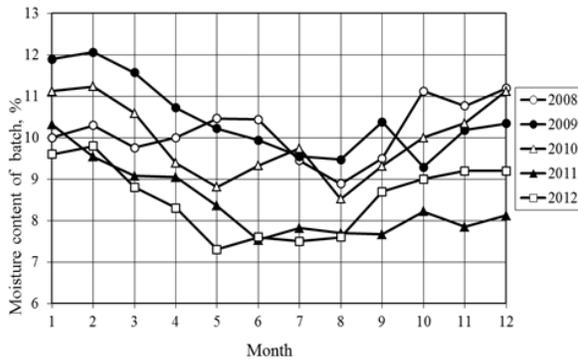
Fig.2. Variation in the moisture content of coal batch at coke batteries 1–4 between 2008 and 2012
