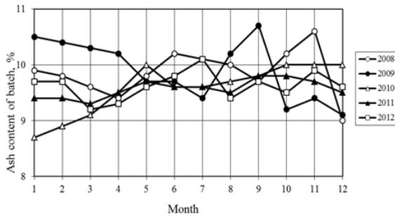
Fig. 3. Variation in the ash content of coal batch at coke batteries 1–4 between 2008 and 2012
