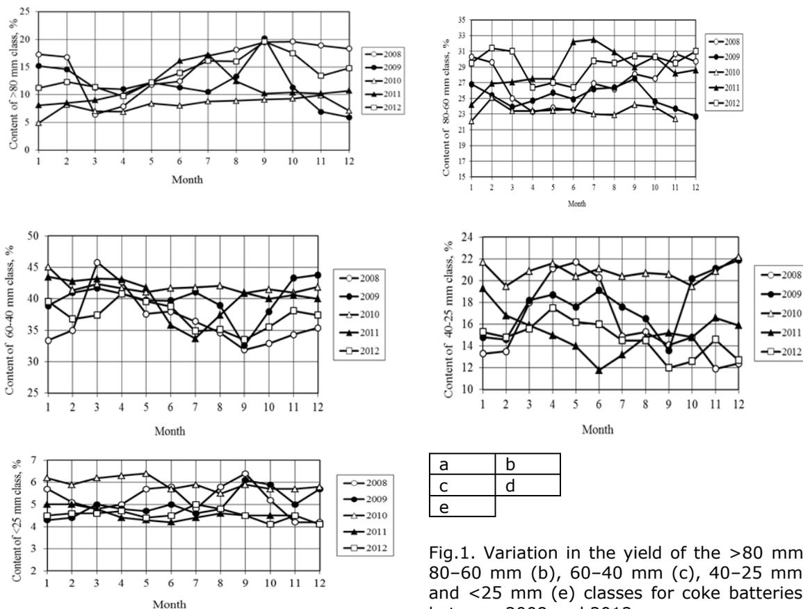
Fig.1. Variation in the yield of the >80 mm (a), 80–60 mm (b), 60–40 mm (c), 40–25 mm (d), and <25 mm (e) classes for coke batteries 1–4 between 2008 and 2012
