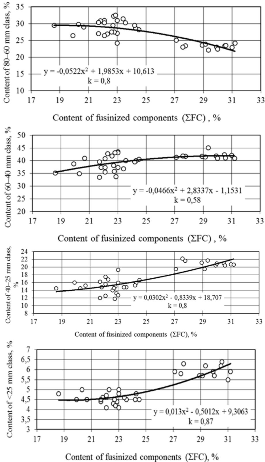
Fig.7. Dependence of the yield of the 80–60 mm (a), 60–40 mm (b), 40–25 mm (c), and <25 mm (d) classes on the content of fusinized components ( $\Sigma FC$ ) in the coal batch at coke batteries 1–4 between 2010 and 2012
