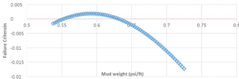
Fig. 3. Failure criterion vs. mud weight for Well T-101
