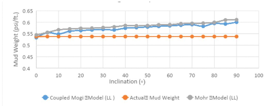
Fig. 8. Comparative analysis of different failure criteria on lower mud density for Well T-101
