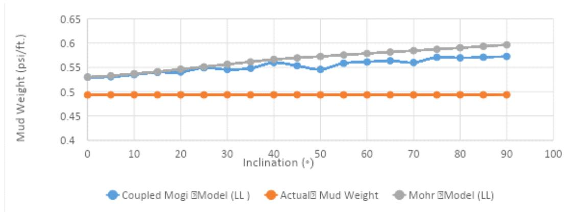
Fig. 10. Comparative analysis of different failure criteria on lower mud density limit for Well A-33
