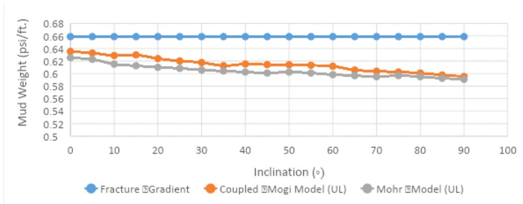
Fig. 9. Comparative analysis of different failure criteria on upper mud density limit for Well T-101
