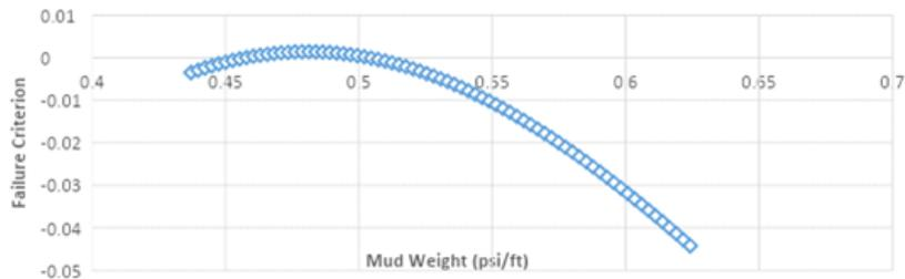
Fig. 7. Failure criterion vs. mud weight for Well Q-01
