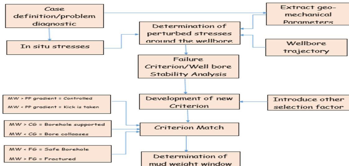
Fig. 2 Workflow for developing suitable criteria for designing sufficient mud weight
