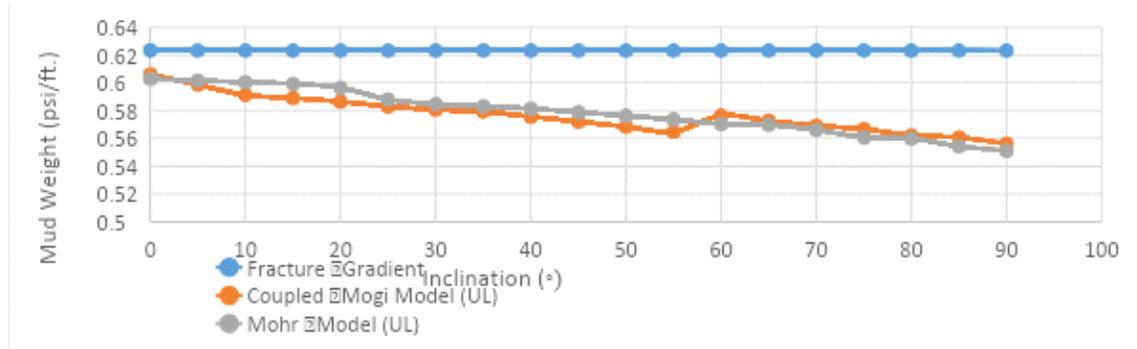
Fig. 13. Comparative analysis of different failure criteria on upper mud density limit for Well D-705
