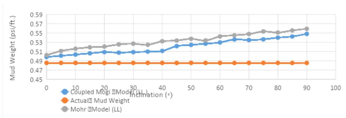
Fig. 12. Comparative analysis of different failure criteria on lower mud density limit for Well D-705
