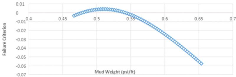
Fig.6. Failure criterion vs. mud weight for Well Z-47
