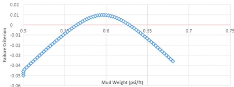
Fig. 4. Failure criterion vs. mud weight for Well A-33
