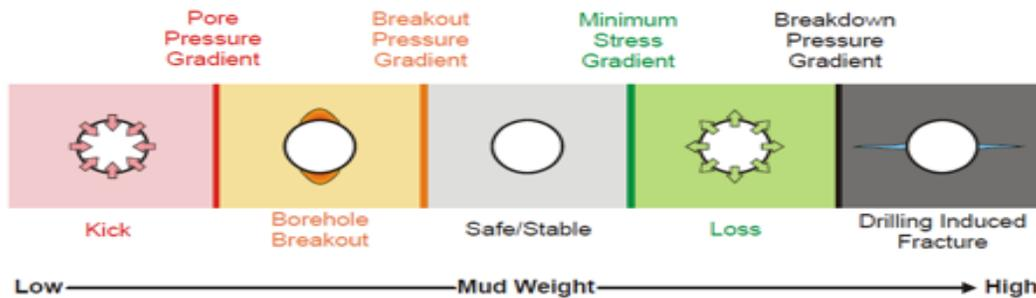
Fig. 1. The concept of safe mud weight Limits for Wellbore drilling [8]
