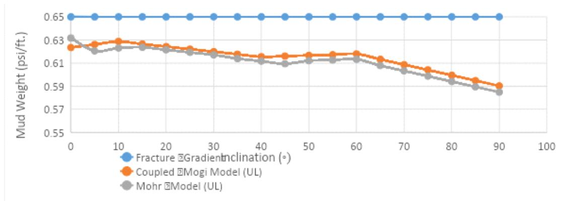
Fig. 11. Comparative analysis of different failure criteria on upper mud density limit for Well A-33
