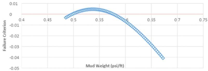
Fig. 5. Criterion vs. mud weight for Well D-705.
