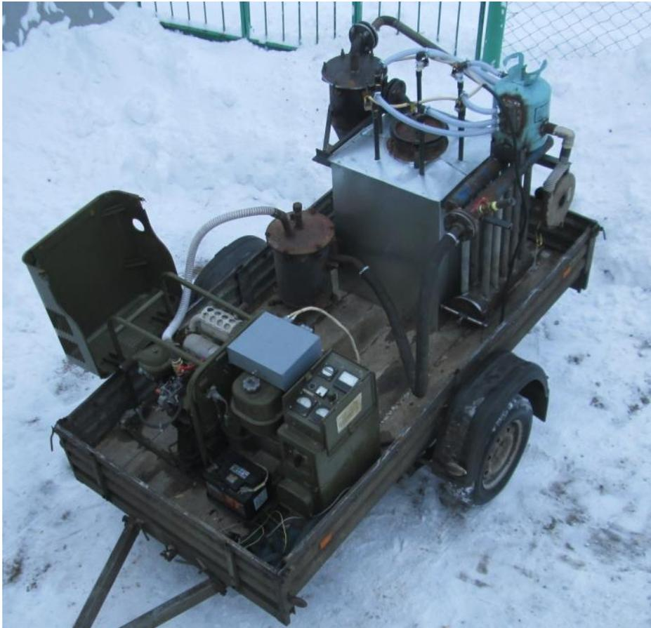
Figure 2. General view of experimental gas generator with ICE 2Ch 7.2/6.0 and electric generator
