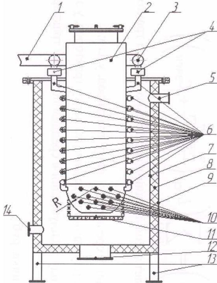
Figure 1. General view of a gas generator: 1 - air pipe, 2 - gasification chamber, 3 - air manifold, 4 - solenoid valve system, 5 - gas outlet pipe, 6 - pipes, 7 - gas tank, 8 - thermal insulation case, 9 - external protective casing, 10 - tuyere belt, 11 - ash grate, 12 - ash pan, 13 - supports, 14 - service hatch, 15 - locking mechanism
