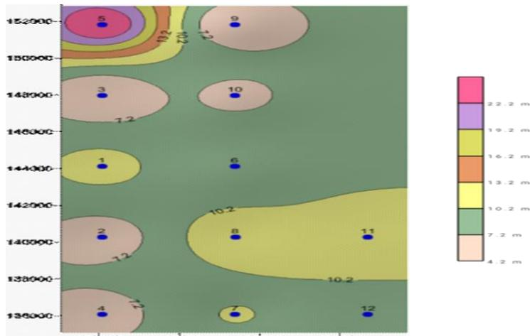
Fig. 10. Weathered Layer Thickness Contour Map
