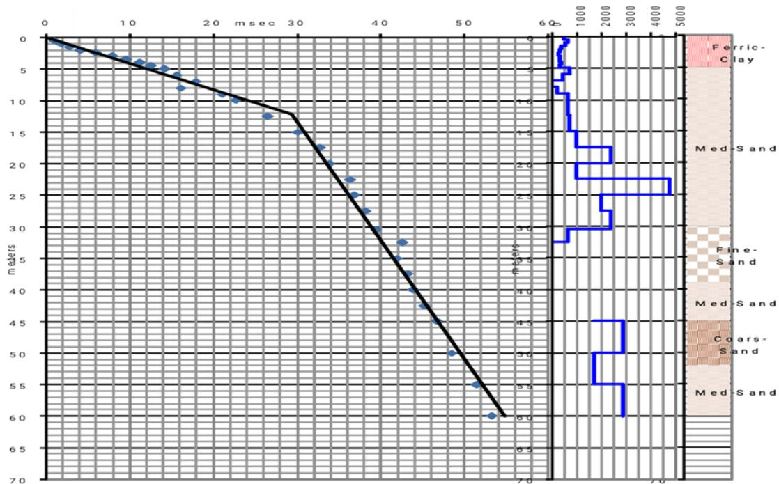
Fig. 8. Distance-time graph of the Uphole Shot at Point 4
