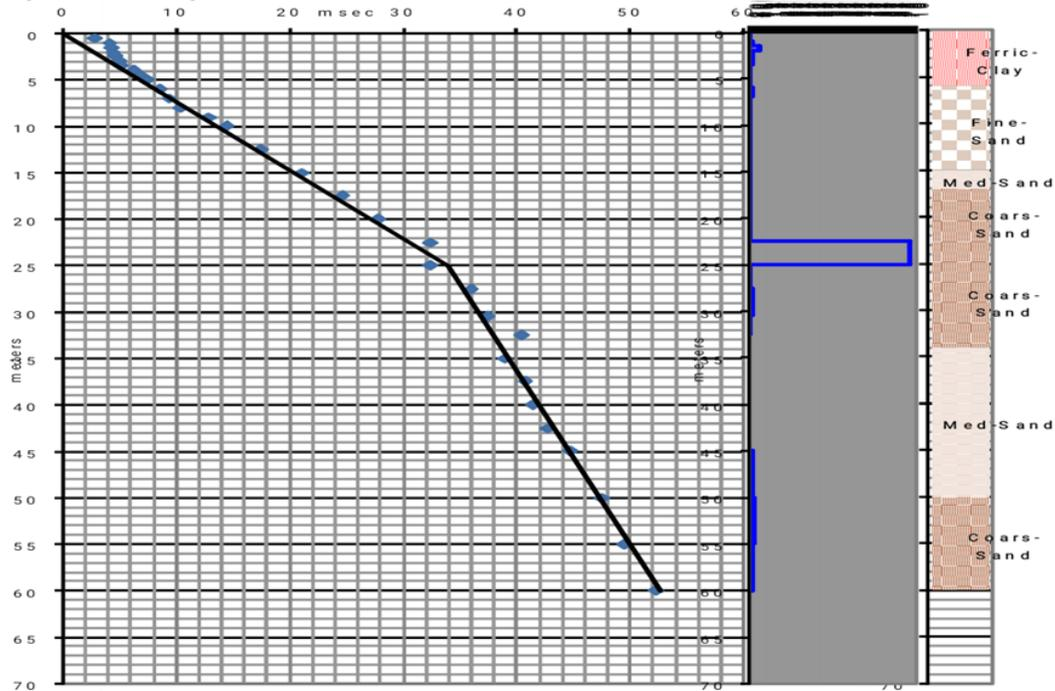
Fig. 6. Distance-time graph of the Up hole shot at Point 1
