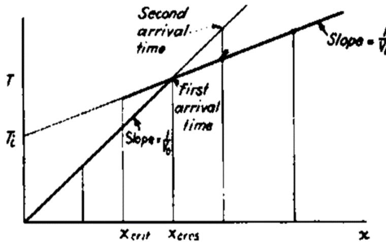
Fig 4b. Schematic diagram illustrating the path of seismic waves
