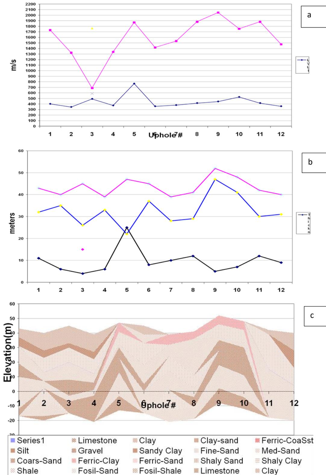
Fig. 14. Cross-sectional plots of the study area showing Up hole Shot points 1 to 12: (a) Cross section showing seismic velocity across the study area (b) Cross section showing elevation across the study area(c) Cross section showing lithology across the study area
