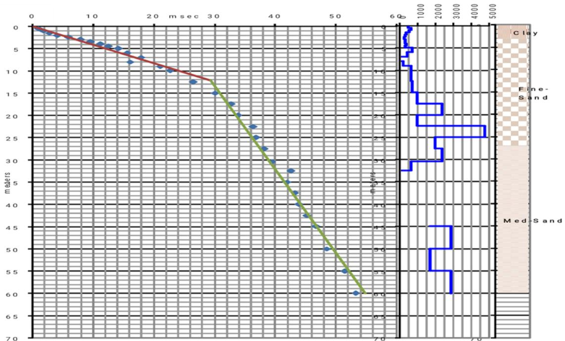
Fig. 7. Distance-time graph of the Up hole Shot at Point 2
