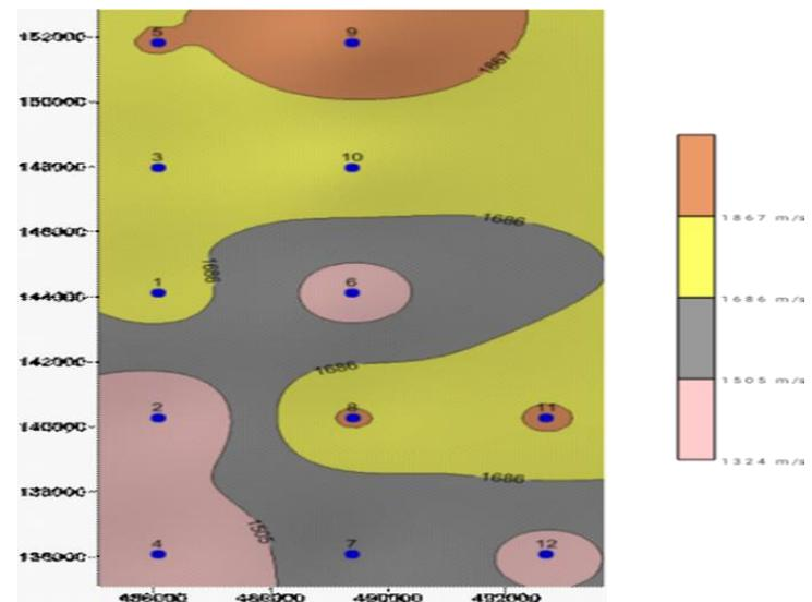
Fig. 12. Consolidated Layer Velocity Contour Map
