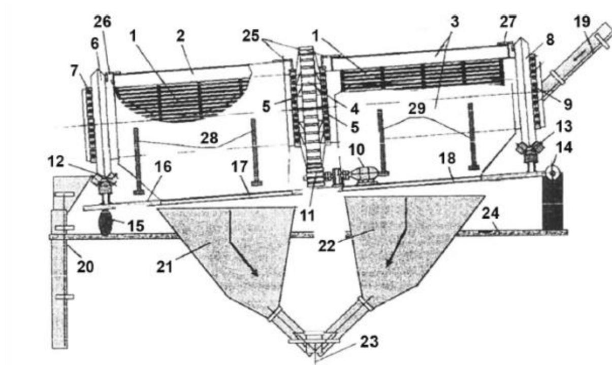
Fig.1. Unit for obtaining the specified properties of coke
