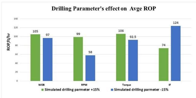
Fig. 6. Sensitivity analysis - Predicted average ROP for increasing/decreasing the different drilling parameters by 15%
