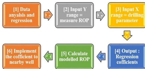
Fig. 2. Multiple regression process flowchart [1].
