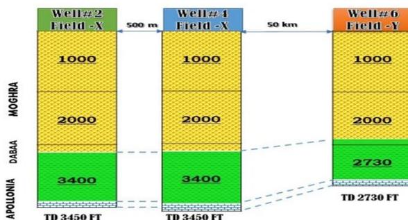
Fig. 4. Stratigraphic correlation between the wells. (not to the scale) [2]
