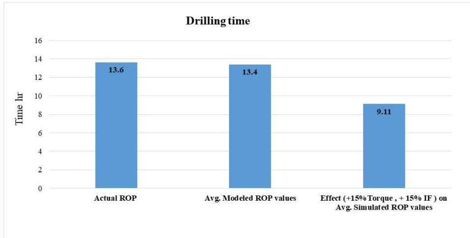
Fig. 10. Amount of time saved after The IF decreased by 15% and the TORQUE increased 15%
