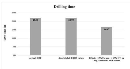
Fig. 7. Amount of time saved after The IF decreased by 15% and the TORQUE increased by 15%
