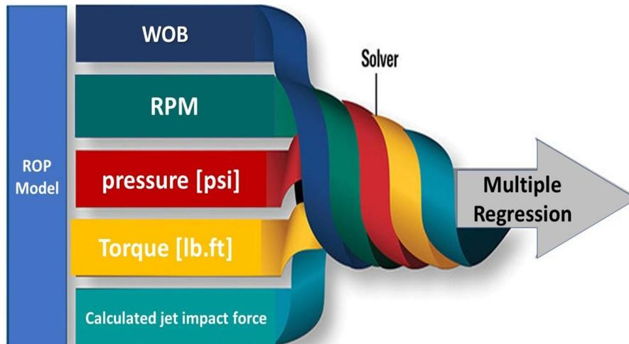
Fig. 3. The input drilling parameter into multiple regression process
