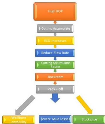
Fig 12. The graphic representation of the high ROP Tap
