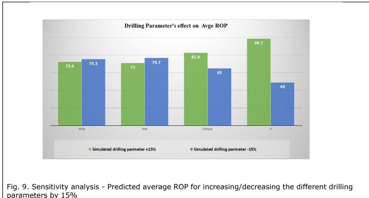
The average ROP of the results is easier to determine the parameters that affect the model most. The IF and the TORQUE are obviously the parameters with the greatest impact on the ROP model in the reference well. This is expected since the corresponding coefficients for
