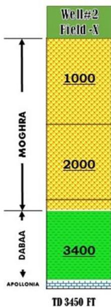
This section presents multiple regression modeling and application. the details of the modeling workflow. Fig. 5 illustrates a sketch of the drilling with casing Well #2 in the field -X (not the scale), which provides perception about the position/shape of the Well. The Fig showed, DwC Well #2 in the field X consists of two main formations in (MOGHRA, DABBA and tagged in APOLLONIA formation by 50 ft. [3]
