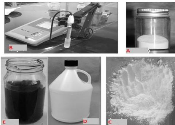
Fig. 4. devices and materials used in clay emulsion preparation: (a) Carboxyl Methyl Cellulose, (b) PH gauge, (c) Sodium carbonate, (d) Dilute sulfuric acid, and (E) image of the clay emulsion prepared using 5% of bentonite emulsifier of type Be1 called S1.50
