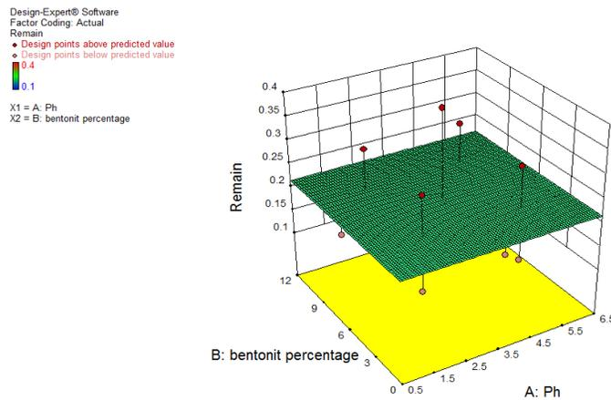
Fig. 6. The plot related to the remained percentages on the sieve 850  $\mu\text{m}$  in terms of bentonite percentage and pH
