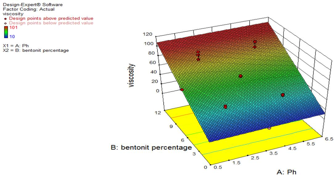
Fig. 5. The plot of the clay emulsion viscosity in terms of the bentonite percentage and pH
