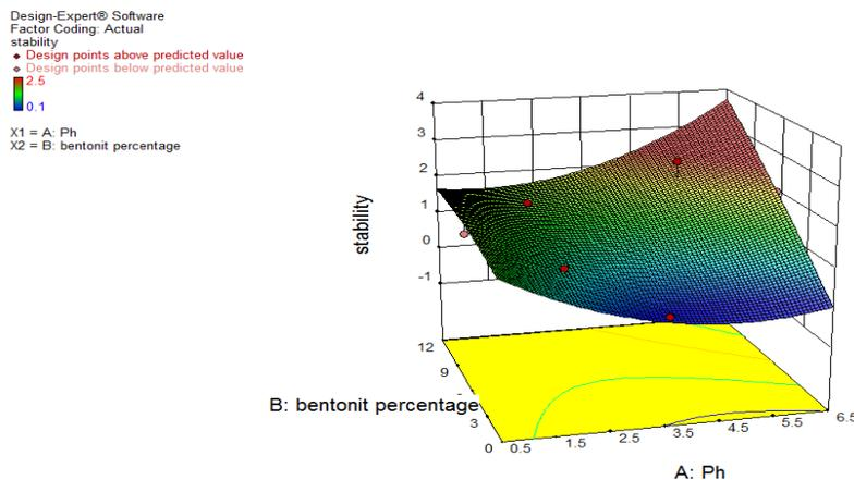
Fig. 7. 24 hours Setting stability test of emulsions for specimens produced of different percentages of bentonites Be1 and Be2
