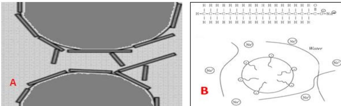
Fig. 1. A photomicrograph of a bitumen emulsion stabilized with (a) clay particles, (b) chemical emulsifier [5-6]
