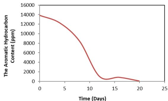
Fig. 4. Aromatic hydrocarbon content biodegradation against time
