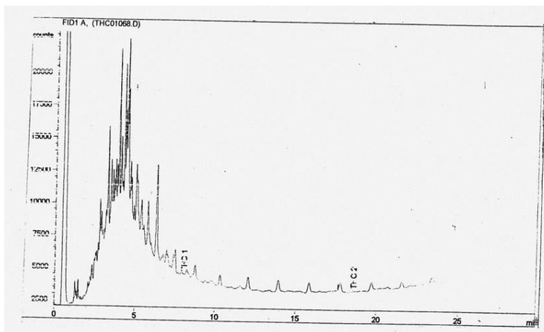
Fig. 2. The GC-FID chromatogram showing the total aliphatic and aromatic hydrocarbon in crude oil after biodegradation
