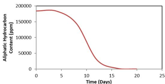
Fig. 3. Aliphatic hydrocarbon content biodegradation against time
