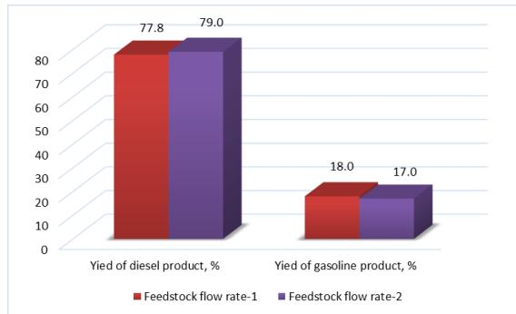
Figure 4. The influence of feedstock flow rate on the product yields in the process of atmospheric oil distillates catalytic dewaxing
