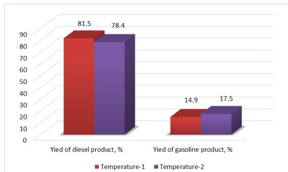
Figure 6. The influence of temperature on the product yields in the process of atmospheric oil distillates catalytic dewaxing
