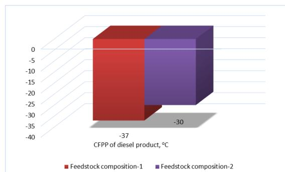
Figure 3. The influence of feedstock composition on the CFPP of diesel product, obtained in the process of atmospheric oil distillates catalytic dewaxing
