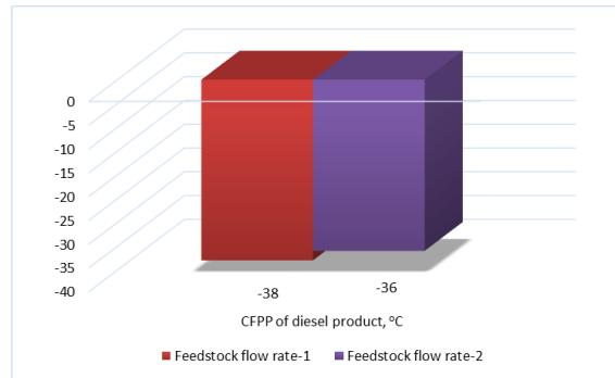
Figure 5. The influence of feedstock flow rate on the CFPP of diesel product, obtained in the process of atmospheric oil distillates catalytic dewaxing
