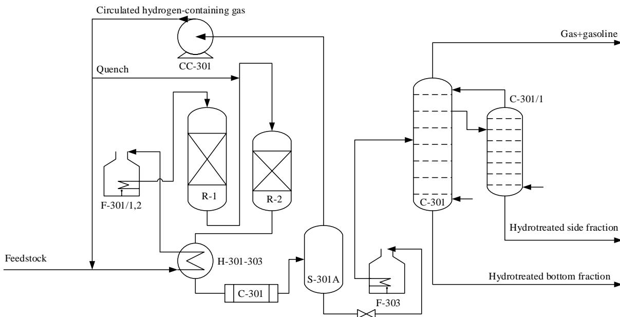
Figure 1. Process flow diagram of the industrial unit for hydrotreating and catalytic dewaxing of atmospheric oil distillates
