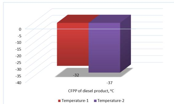
Figure 7. The influence of temperature on the CFPP of diesel product, obtained in the process of atmospheric oil distillates catalytic dewaxing
