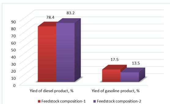
Figure 2. The influence of feedstock composition on the product yields in the process of atmospheric oil distillates catalytic dewaxing
