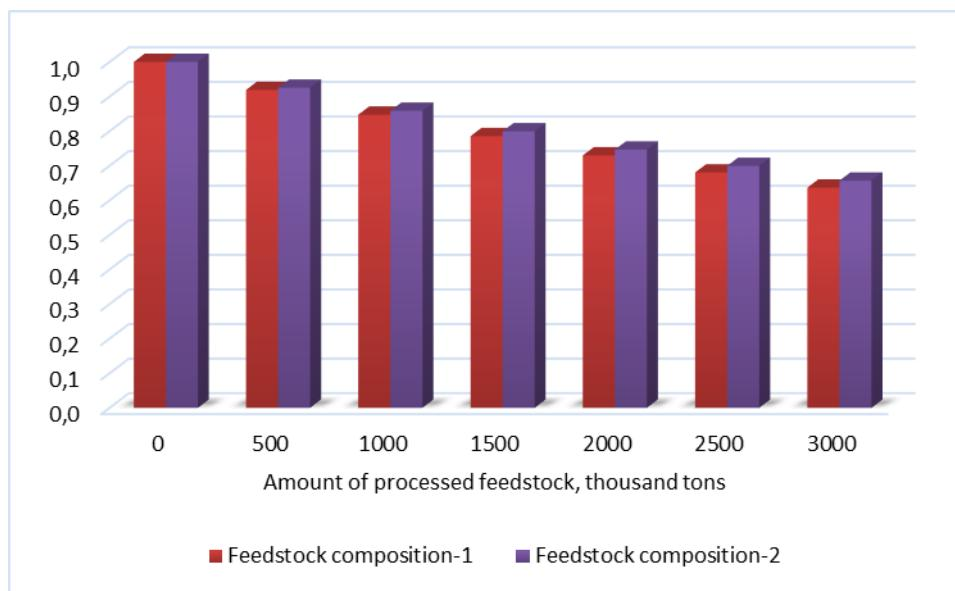
Figure 8. Prognostic calculation on the changing in relative catalyst activity in the process of atmospheric oil distillates dewaxing
