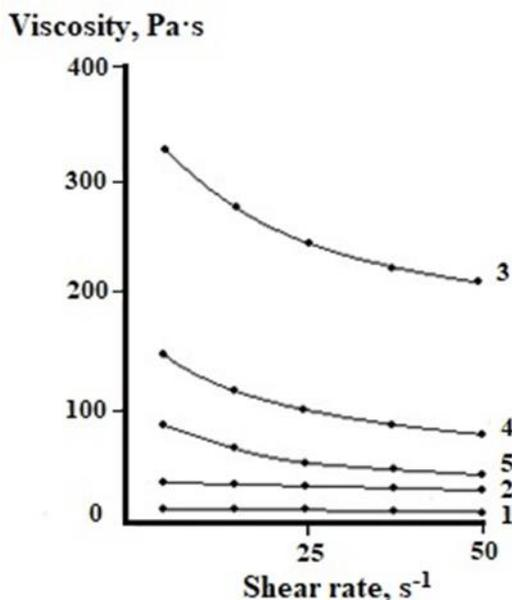
Figure 5. The dependence of viscosity (at  $135^{\circ}\text{C}$ ) on the shift speed of CTP and pitches, modified with 3 wt.p. of PVC: 1 – initial pitch; 2 – pitch, heat-treated without additives; 3 – pitch, modified at  $135^{\circ}\text{C}$ ; 4 – pitch, modified at  $145^{\circ}\text{C}$ ; 5 – pitch, modified at  $155^{\circ}\text{C}$
