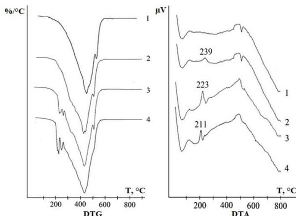
Figure 3. DTG and DTA curves of CTP, modified with PVC at 170 °C for 120 min. PVC amount: 1 – 0 wt.p.; 2 – 1 wt.p.; 3 – 3 wt.p.; 4 – 5 wt.p.
