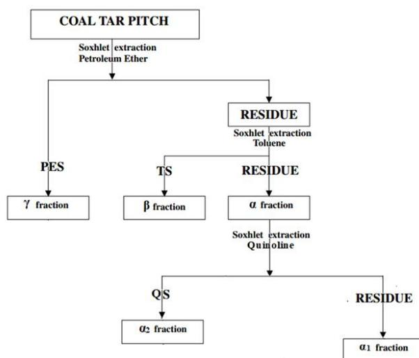
Figure 1. Scheme for the separation of the initial and modified pitches (PE – petroleum ether; T – toluene; Q – quinoline)
