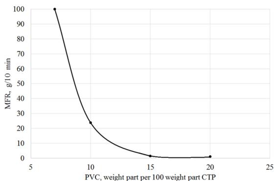
Figure 6. Dependence of the MFR of the modified pitch on the amount of PVC (load weight 10 kg at 150°C)
