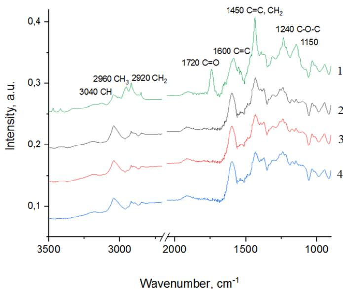
Figure 4. FTIR spectra of CTP (1) and pitch modified with PVC at 170°C for 120 min. Amount of PVC: 2 – 5 wt.p.; 3 – 10 wt.p.; 4 – 20 wt.p.
