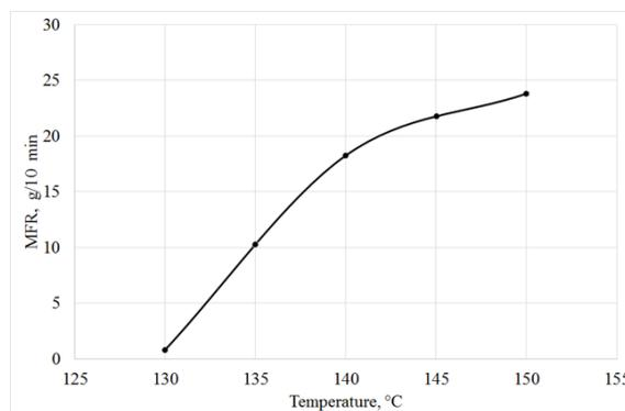
Figure 7. Dependence of the MFR of pitch modified with 10 wt.p. of PVC (load weight 10 kg) on the temperature
