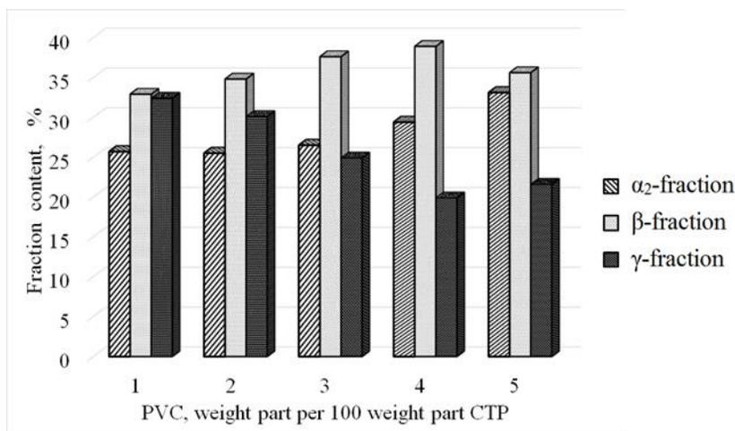
Figure 2. Group composition of the CTP, heat-treated without additives, and CTP modified with PVC (at 170 °C for 120 min)
