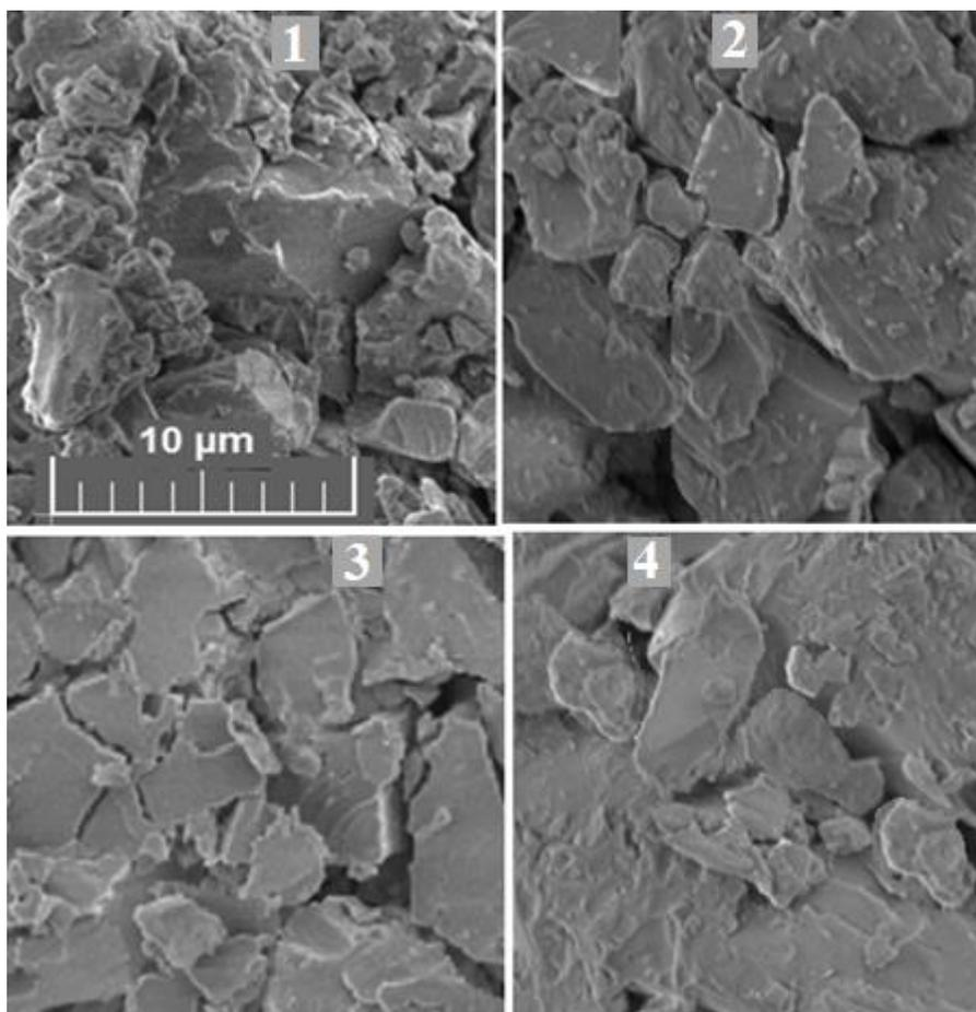
Figure 10. SEM micrographs of samples of the initial (1) and modified pitch. The amount of PVC: 2 – 5 wt.p.; 3 – 10 wt.p.; 4 – 20 wt.p.
