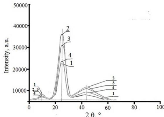
Figure 9. Corrected XRD diffractogram of initial and modified pitches. The corrected profiles of diffraction peaks (002), (10) and  $\gamma$ -band of the initial pitch (1) and pitches modified with PVC: 2 – 5 wt.p.; 3 – 10 wt.p.; 4 – 20 wt.p.
