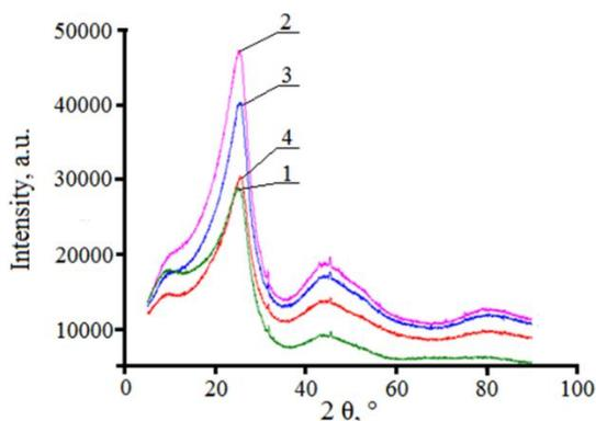
Figure 8. Initial XRD diffractogram of initial and modified pitches. Experimental profiles of diffraction peaks (002), (10) and  $\gamma$ -band of the initial pitch (1) and pitches modified with PVC: 2 – 5 wt.p.; 3 – 10 wt.p.; 4 – 20 wt.p.
