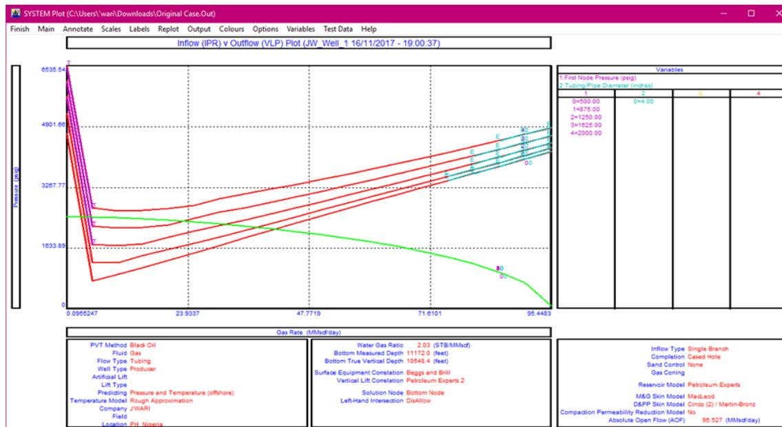
Fig. 5. System plot showing various wellhead pressures for a 4 in. tubing
