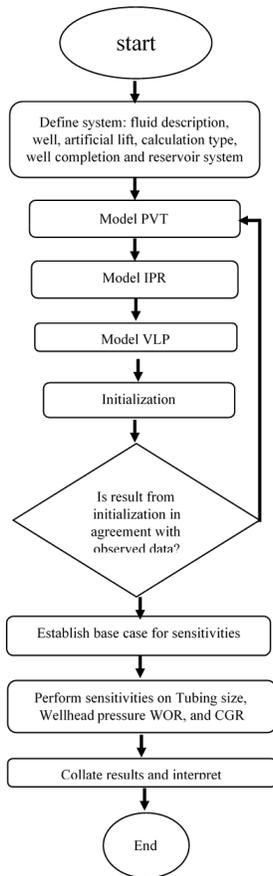
The principle of Nodal Analysis was used to investigate four parameters: tubing size, well head pressure, condensate-gas ratio and water-oil ratio to determine their impacts on liquid accumulation in gas wells using PROSPER. This was achieved using data from Niger Delta.
