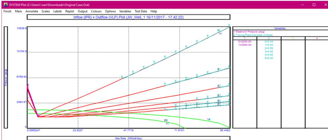
Fig. 4. VLP/IPR matching showing various tubing sizes
