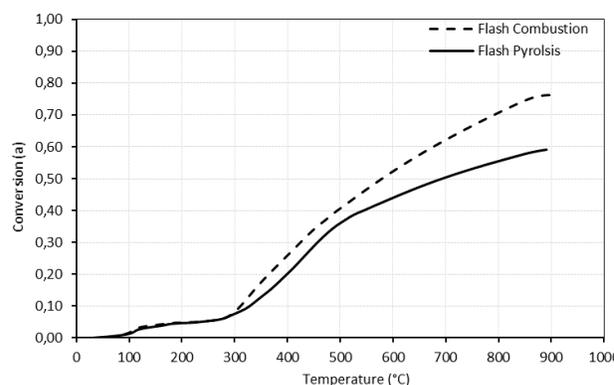
Figure 2. Conversion plots for flash conversions of BMK
