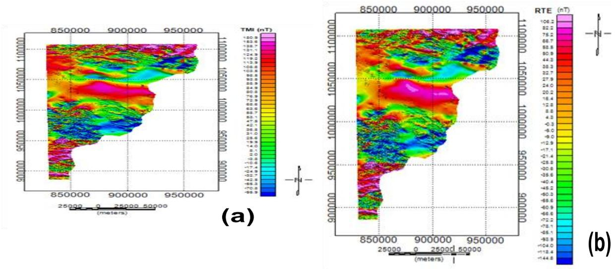
Fig. 2a and b. Total magnetic intensity and residual maps of the study area respectively
