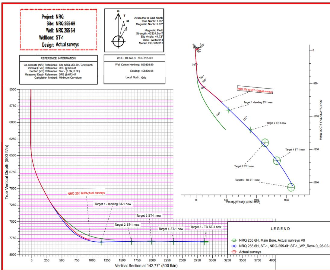
Figure 6. Actual horizontal well trajectory- the planned versus the reality [10]
