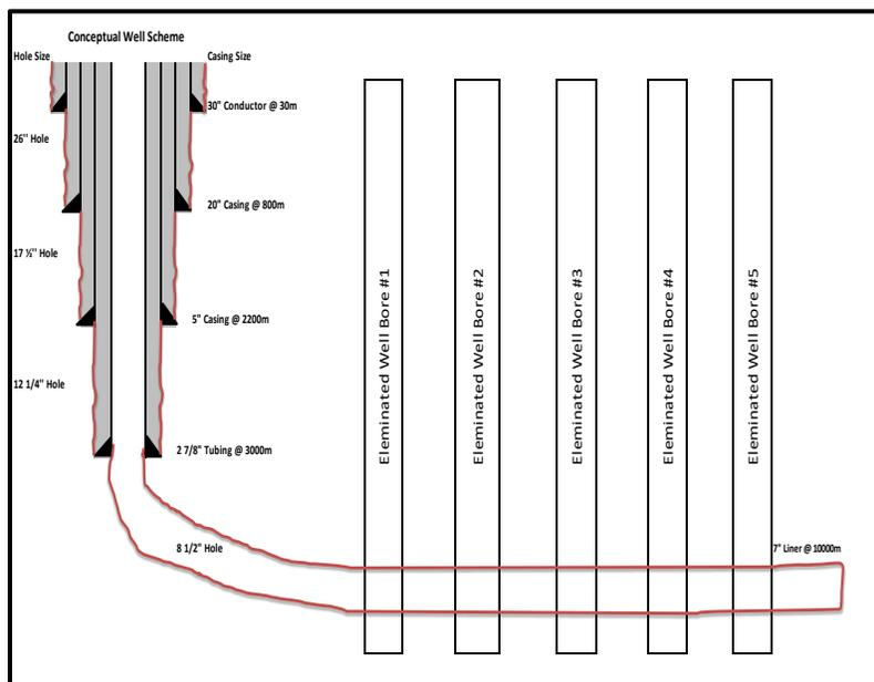
Figure 5. Conceptual Well Scheme for an ERD Project
