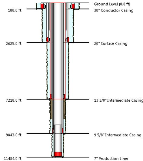
Figure 2. A typical well scheme for a conventional well
