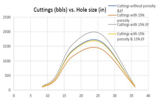
Figure 4. Amount cuttings generated in conventional well
