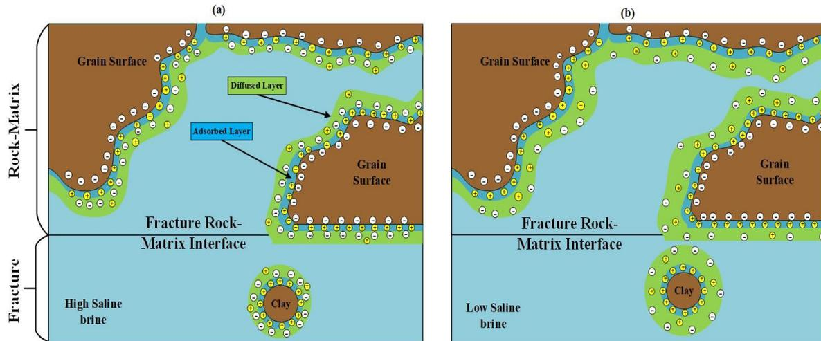
Fig. 3. Impact on the electrical double layer expansion (a) Before LSWF near the IW with high saline formation water (b) Expansion of double layer due to LSWF in a coupled fracture-matrix system
