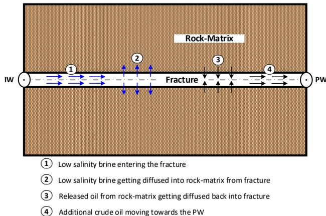
Fig. 1. Conceptual model of LSWF mechanism in a fractured reservoir using dual-porosity approach
