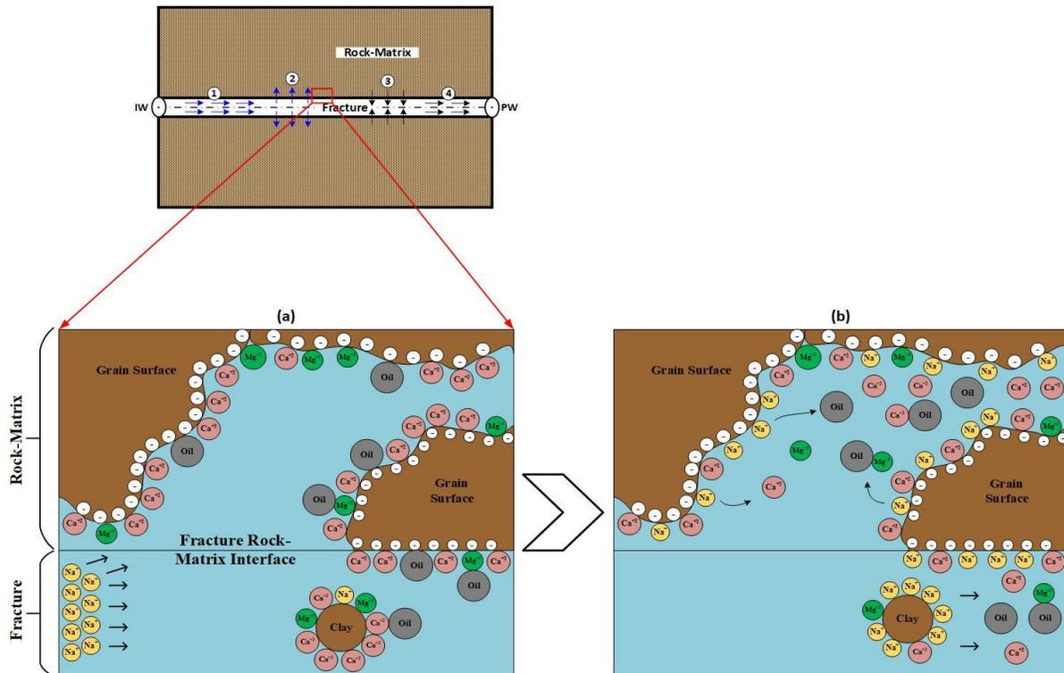
Fig. 2. Multicomponent ion exchange phenomenon in a coupled fracture-matrix system (a) before the injection of low saline brine near the Injection Well (IW) and (b) after the injection of low saline brine towards the production well
