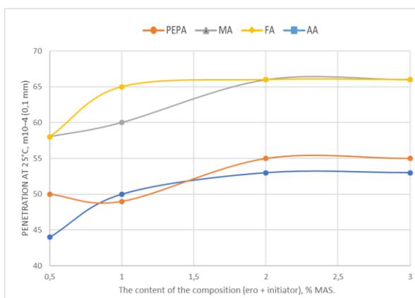
Figure 4. Dependence of penetration of modified bitumen on the content of the composition [EPO: initiator]
