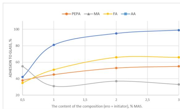
Figure 3. The dependence of the adhesion of the modified bitumen on the content of the composition [EPO: initiator]
