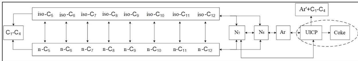
Figure 2. Formalized reaction scheme of naphtha reforming: n-C<sub>n</sub>, iso-C<sub>n</sub> – normal and iso-alkanes; N-5, N-6 – methylcyclopentane and methylcyclohexanes; Ar – aromatic hydrocarbons; UICP – unsaturated immediate compacting products
