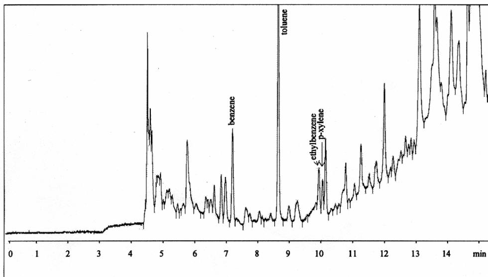
**Figure 3.** Chromatogram from the analysis of 200 ml air sample from town crossroad.
