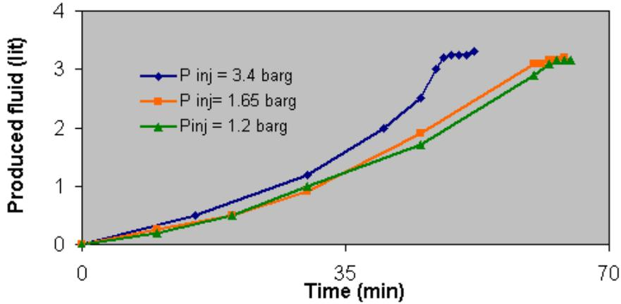
Figure (4): Produced Fluid versus Time (Sample No. =2)
