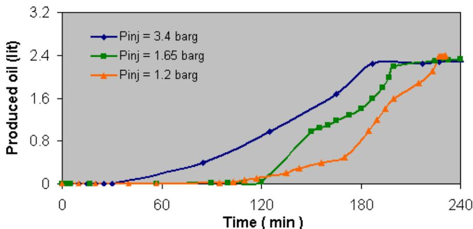
Figure (3): Produced Oil versus Time (Sample No. 1)
