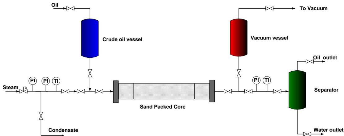
Figure (1): Steam injection set up
