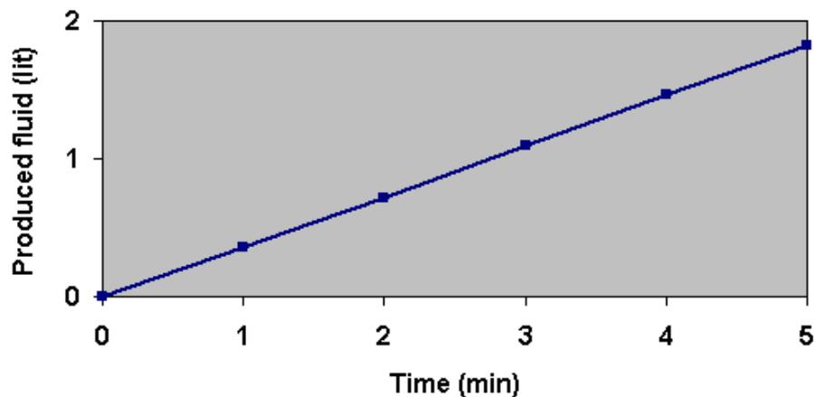
Figure (8): Produced Oil versus Time cold water injection
