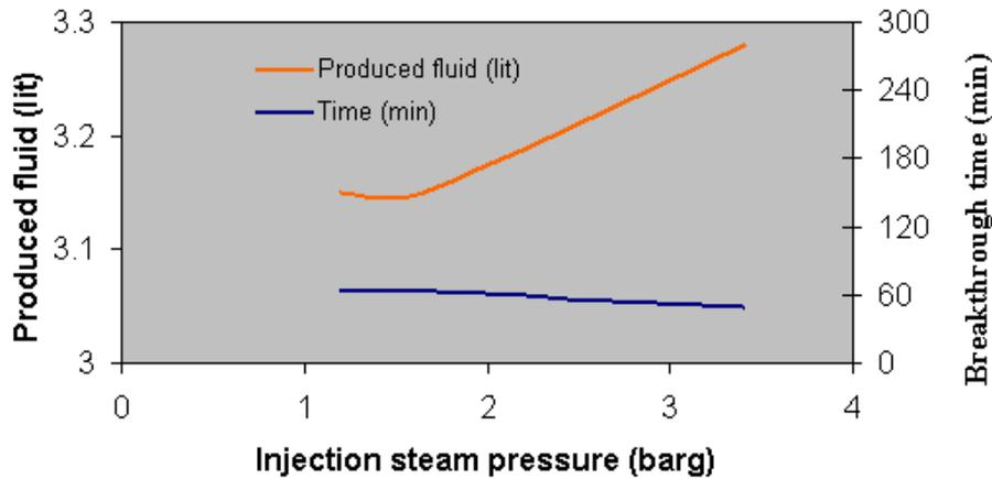
Figure (7): Breakthrough point curve (Sample No. =2)
