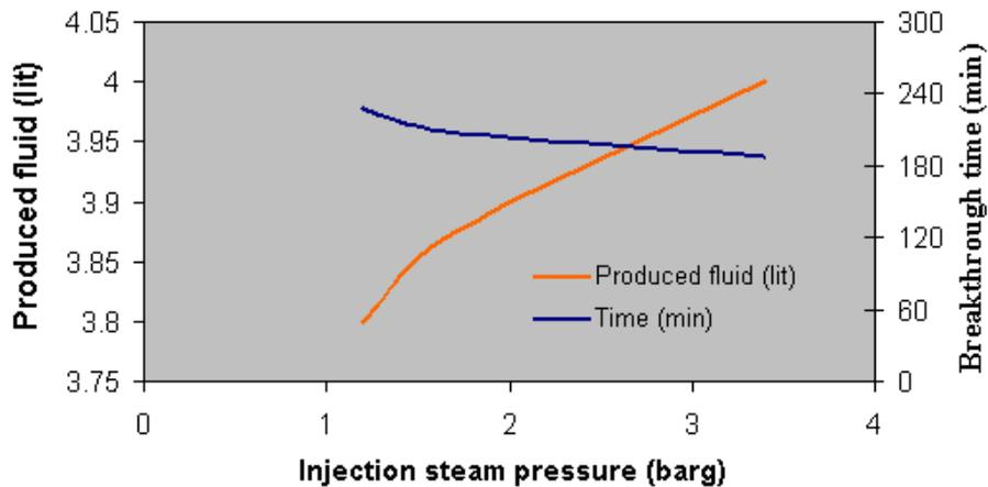
Figure (6): Breakthrough point curve (Sample No. =1)
