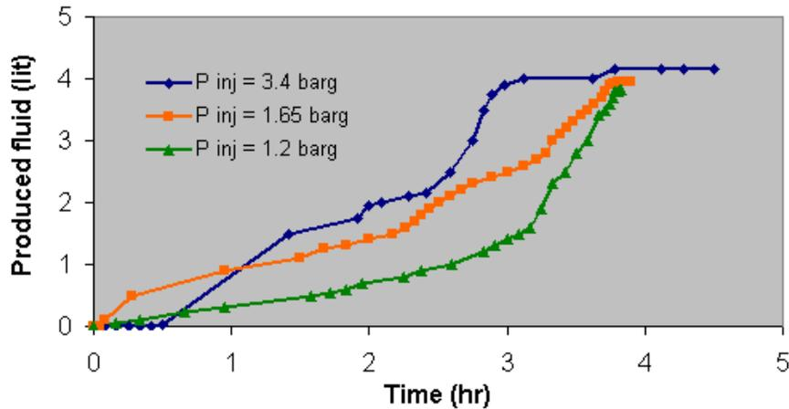
Figure (2): Produced Fluid versus Time (Sample No. =1)
