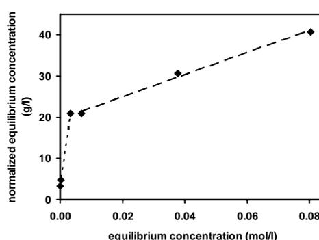
Fig. 4: Adsorption isotherms for the fluoride sorption on lignite from the NaF solutions in the linearized Langmuir coordinates
