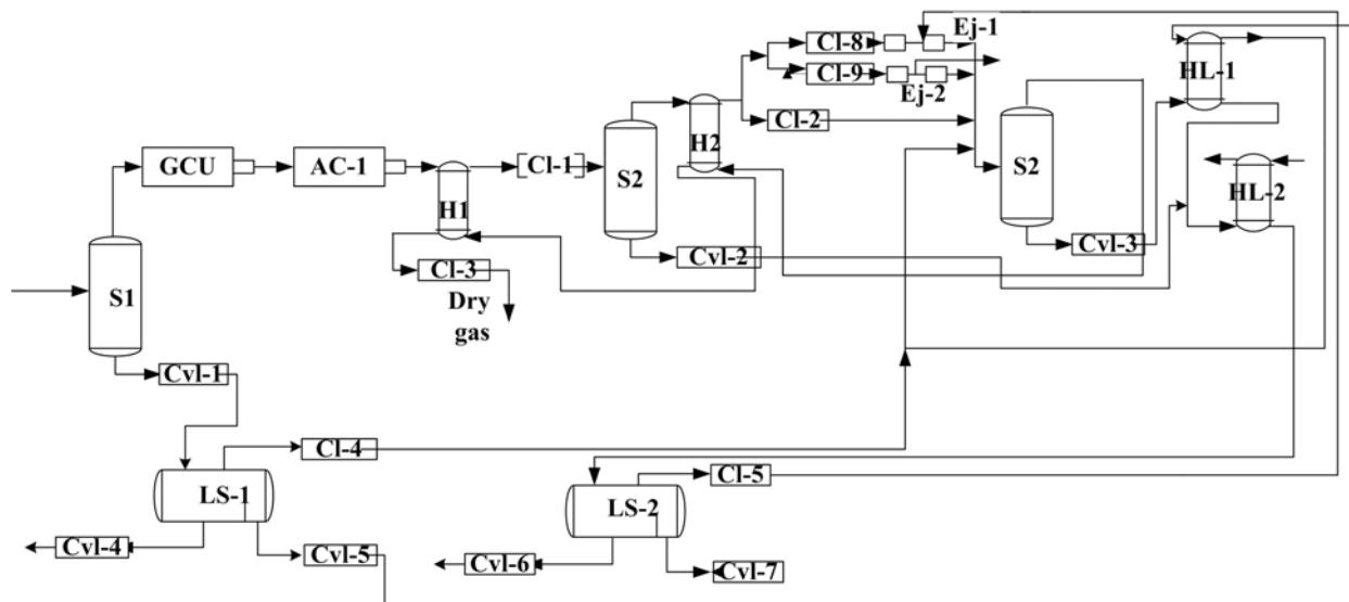
Figure 1. Technological scheme of gas treatment by low-temperature separation: S-1, S-2, S-3 - vertical gas separators; H1, H2 - heat exchangers such as "gas-gas", TL-1, TL-2 - type heat exchangers "liquid-liquid"; LS-1, LS-2 - three-phase separators - liquid separators; Cv-1, Cv-2, Cv-3, Cv-4, Cv-5 - control valves for gas; Cv1-1, Cv1-2, Cv1-3, Cv1-4, Cv1-5, Cv1-6, Cv1-7 – control valves for liquid; GCU - gas compressor unit - gas turbine; AC-1 - air cooler; Ej-1, Ej-2 - gas ejectors.
