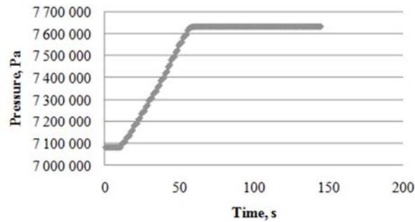
Fig. 4. Dependence of pressure in separator on time
