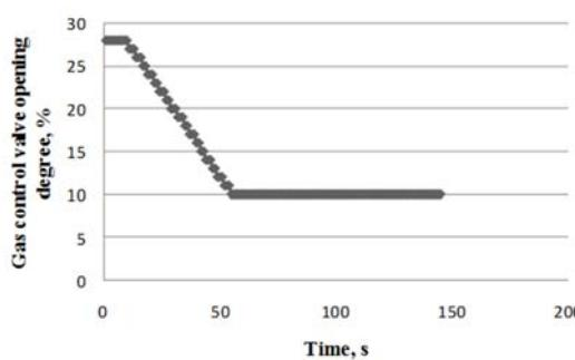
Fig. 3. Changes of gas control valve opening degree against time (manual control)
