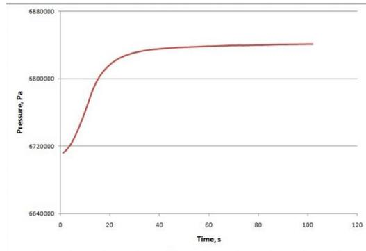
Figure 14. Pressure stabilization in second stage separator during certain time with quarter-opened valve
