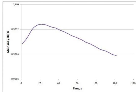
Figure 16. Methane yield in thermodynamic conditions of quarter-opened valve
