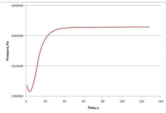
Figure 10. Pressure stabilization in second stage separator during certain time with half-opened valve
