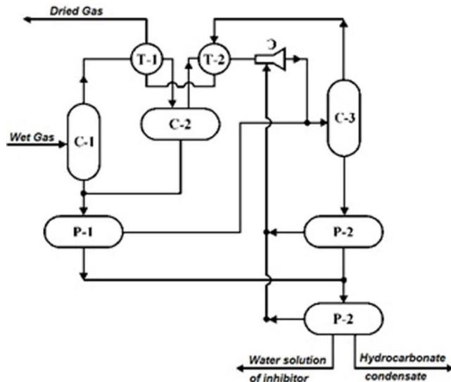
Figure 1. Low-temperature separation scheme
