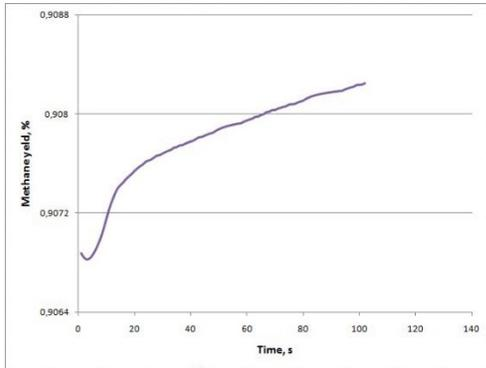
Figure 12. Methane yield in thermodynamic conditions of half-opened valve
